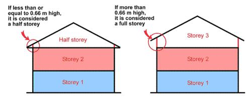
Under Section 6.1(98), **Storey** means that portion of a building, which is situated between the top of any floor and the top of the floor next above it. If there is no floor above, the Storey is the portion of the building, which is situated between the top of any floor and the ceiling above it. If the top of the floor directly above a Basement is more than 1.83 metres above grade, such Basement shall be considered a Storey for the purpose of this Bylaw;
