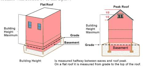
Under Section 6.1(47), **Half Storey** means a Storey under a gable, hip, or gambrel roof, the wall plates of which, on at least two opposite walls, are not more than 0.66 metres above the floor of such Storey;
