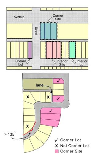
Under Section 6.1(90), **Side Setback** means the distance that a development or a specified portion of it, must be set back from a Side Lot Line. A Side Setback is not a Side Yard, Amenity Space or Separation Space.
